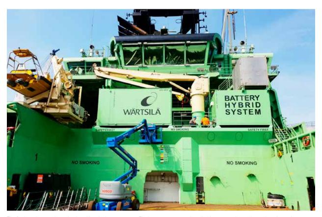
The final touches are done after installing the battery system: The battery system was installed in two containers; the starboard container includes the batteries and the port container, the power converter.
