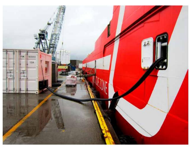
Shore connection cables connected at Mongstad base, supplying electric power to the ship while moored at quay
