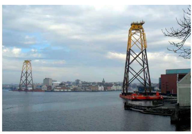
Transport of jackets for windmills; barge UR 99 to the left and barge UR 901 to the right
